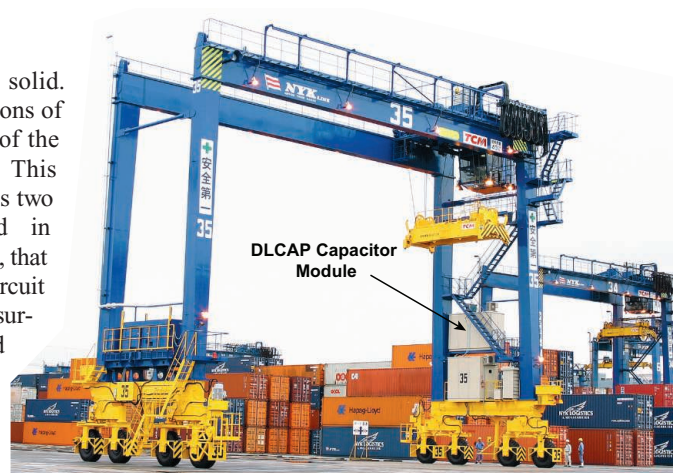
ECs at work. Hybrid diesel/electric rubber-tired gantry crane with DLCAP electrochemical capacitor energy storage system (fuel savings of 40% are typical).
